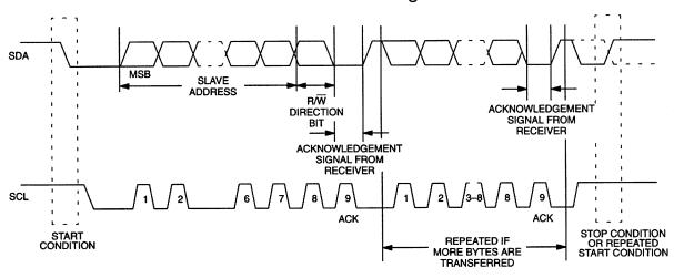
Figure 4 details how data transfer is accomplished on the 2-wire bus. Depending upon the state of the R/W bit, two types of data transfer are possible:
