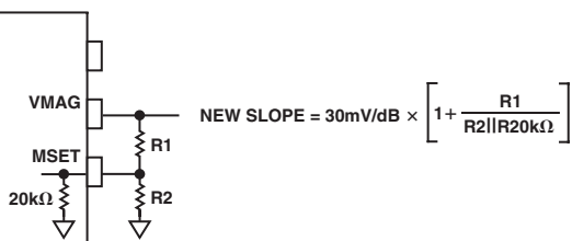
Figure 8. Increasing the Slope Requires the Inclusion of a Voltage Divider
