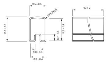
Tube for SMT version - 40 relays per tube 2000 relays per box
