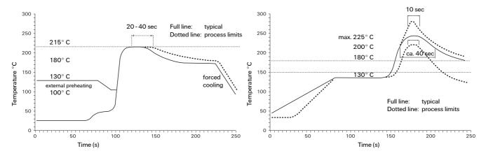
Vapor Phase Soldering: Temperature/Time Profile (Lead Temperature)
