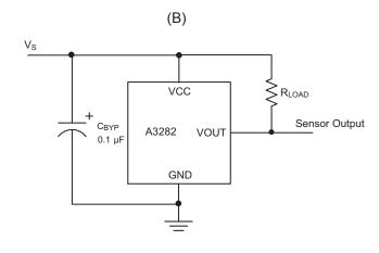
Figure 1: Switching Behavior of Latches. In Panel A, on the horizontal axis, the B+ direction indicates increasing south polarity magnetic field strength, and the B- direction indicates decreasing south polarity field strength (including the case of increasing north polarity). This behavior can be exhibited when using a circuit such as that shown in panel B.
