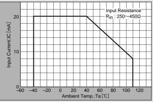
Note :  $R_{\text{in}}$  of Hall element decreases rapidly as ambient temperature increases. Ensure compliance with input current derating curve envelope, throughout the operating temperature range.
