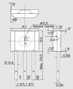
Note1) The sensor center is located within the  $\phi$ 0.3mm circle. Note2) The metal portions on the package side (support lead) are connected to the internal circuits. The support lead should be isolate from the external circuit and the other support lead.
