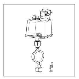
To protect the pressure element against excessive temperature of the media, above allowable 120 °C the insertion of water-filled loop is recommended.
