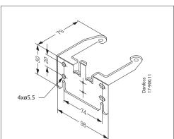
Mounting bracket for T 35 mm rail, code number 017B1019
