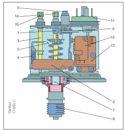
Version with automatic reset cut-in again automatically when the pressure falls to the set point minus differential. Version with manual reset has to be cut in manually by means of tool.
