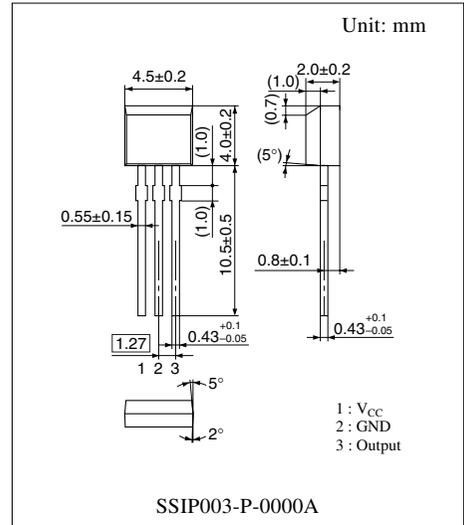
Note) The package of this product will be changed to lead-free type (SSIP003-P-0000H). See the new package dimensions section later of this datasheet.
