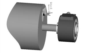
**STEP 5:** While making sure not to disturb the position of the flex mount, slide encoder off the shaft and tighten the mounting bolt firmly.
