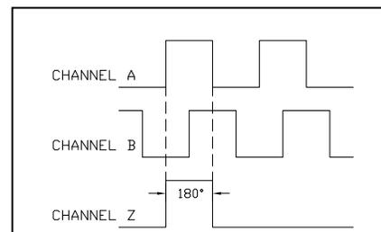
**Figure 4.** Quadrature encoder with an index channel.
