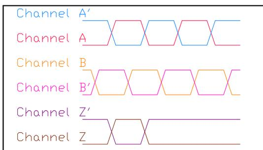
Figure 5. Differential outputs.
