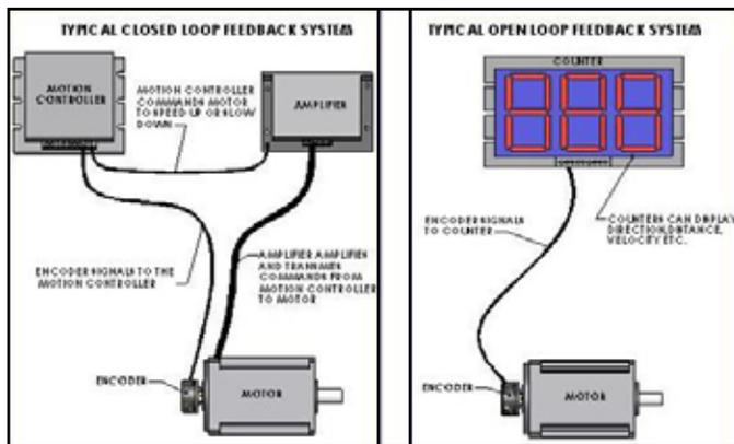
**Figure 1.** Two types of feedback systems. Closed loop feedback is where the encoder signals control the motor without any user inputs. Open loop feedback is where the encoder signal runs to a display and the user adjusts the motor to fit a desired output.
