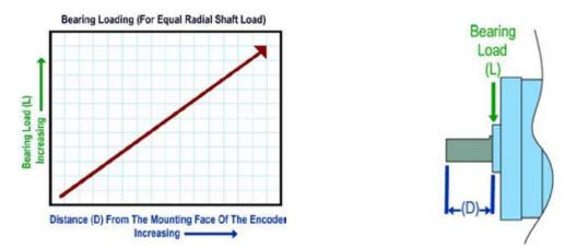
If a flexible coupling, belt or chain is applied to the encoder shaft, ensure that **proper alignment** is maintained to minimize axial loads. Likewise, a measuring wheel that engages the measured surface at an angle will exert radial and possibly axial loads on the encoder shaft.
