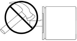
Also, with shaft encoders, it is important to utilize a flexible shaft coupling. Rigid couplings can transmit harmful inputs to the encoder shaft and the bearings such as vibration, shaft end run-out, misalignment or other loads. EPC offers a number of industry standard <u>shaft</u> <u>couplings</u> as accessories. For more complete details on proper encoder installation, see our <u>Encoder Installation and Wiring Guide</u>.
