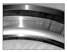
surface material is heated to temperatures ranging from tempering to melting levels. This leads to the appearance of discolored areas, varying in size, where the material has been tempered, re-hardened or melted. Small craters also form on the bearing surface where the metal has melted.
