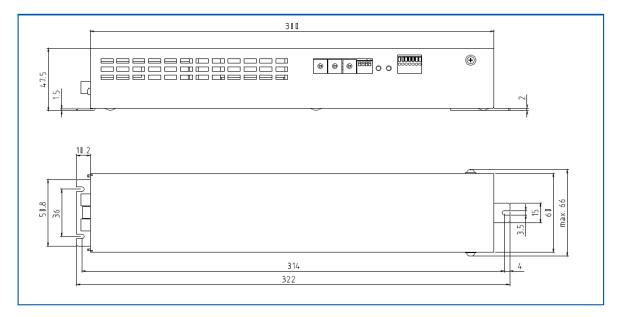
Figure 1 Dimensions of the DMX power supply
