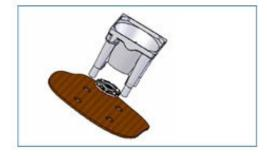
Do not look directly into the high-power LED light source. The high intensity beam could cause irreversible damage to your eyes. Figure 5 How to assemble lens (holder), ACULED and substrate (heat sink) in principle.
