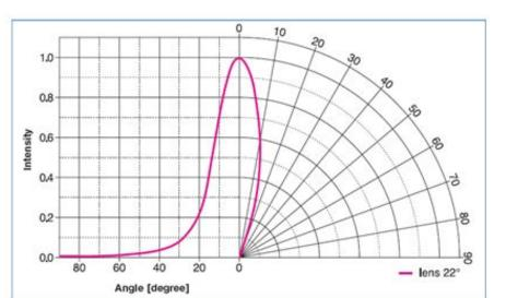
Figure 3 Opening Angle: Example RGB with Lens
