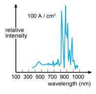
Spectrum of a high impedance flashtube
