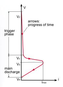
The impedance characteristic of the flash discharge
