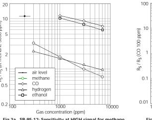
Fig 3a. SB-95-12: Sensitivity at HIGH signal for methane
