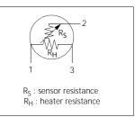
Fig 1c. Pin Layout
