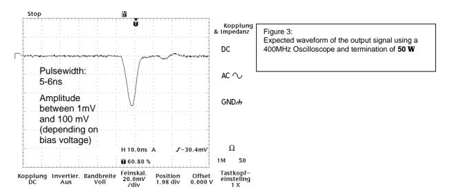
The signal of a Channel Photomultiplier can be operated either in analogue dc mode, in photon counting mode or in pulse mode (not discussed here)
