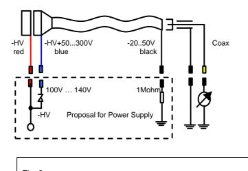
Fig. 8 Typical application circuit when using a *negativ*e high voltage supply (0 to – 3000 volts)
