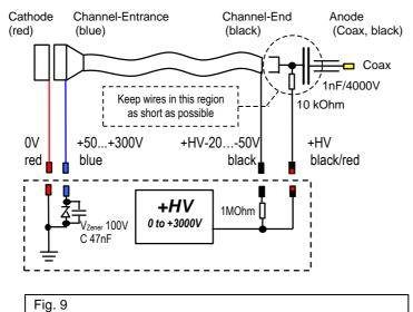
Typical application circuit when using a *positive* high voltage supply (0 to + 3000 volts)
