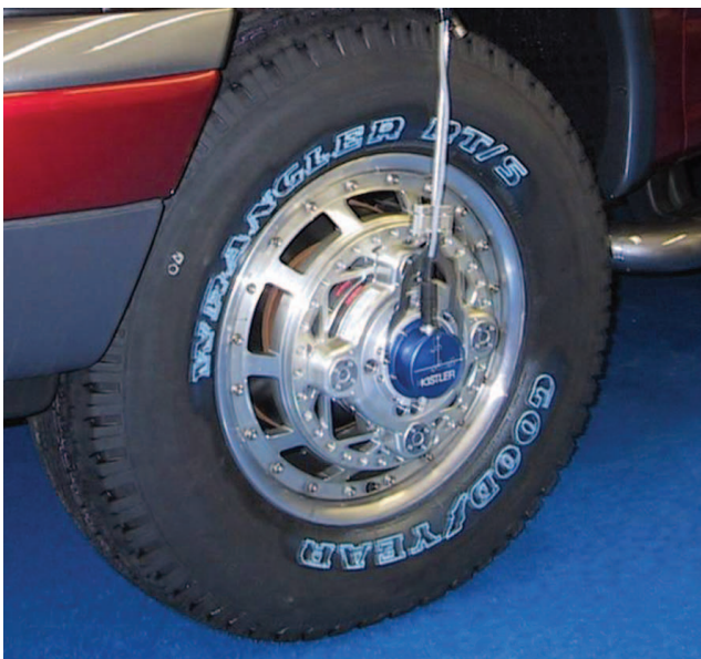
Fig. 4: RoaDyn® P650 analog mounted at front axle
