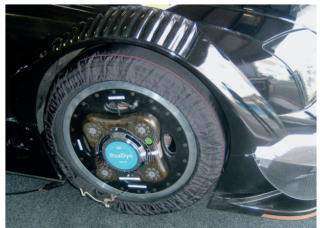
Fig. 2: Race car with RoaDyn® S625 System 2000
