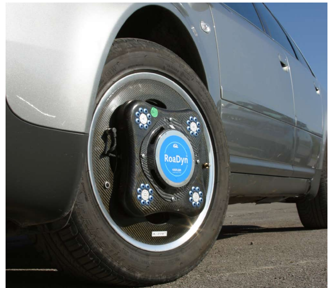
Fig. 1: Passenger car with RoaDyn® S625 System 2000
