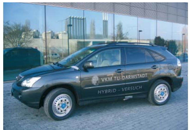
Fig. 2: RoadDyn® P106 on hybrid vehicle
