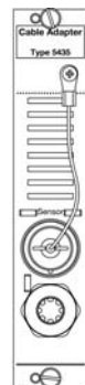
Fig. 15: Cable adapter plate Type 5435Ax, input Fischer 9-pole neg. and output BNC pos.
