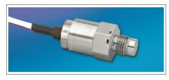
for operation from an unregulated power supply ranging from 12  $\pm$  4VDC or 28  $\pm$  4VDC with reverse polarity protection available upon request. The result is a stable, digitally corrected 0 to 5 VDC output signal.
