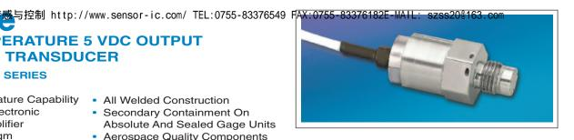
influence on the frequency response of the sensor. For applications where a true flush diaphragm is needed, Kulite will supply these transducers without the screen. Incorporation of a Kulite proprietary electronics module within the main body of this product allows for operation from an unregulated power supply of 12 ± 4 VDC or 28 ± 4 VDC. Standard output is a stable, low noise 0 to 5 VDC signal.
