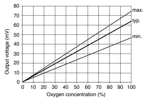
Fig. 3a - KE-25 sensitivity characteristics
