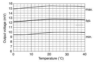
Fig. 8a - KE-25 temperature dependency of output voltage
