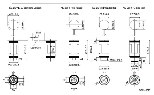
Figure 2 - Dimensions of KE-25/KE-50
