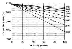
Fig. 7 - Effect of humidity on O2 concentration
