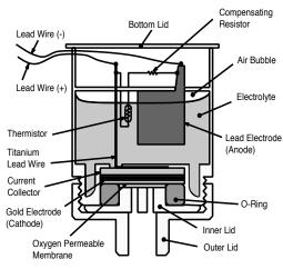
Fig. 1 - Structure of KE-25/KE-50
