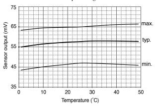
Fig. 8b - KE-50 temperature dependency of output voltage
