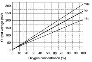
Fig. 3b - KE-50 sensitivity characteristics
