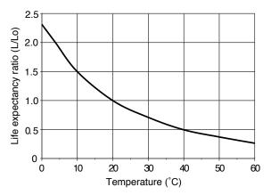
Fig. 9b - Relationship of life expectancy vs. temperature (Lo = life at  $20^{\circ}$ C)
