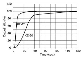
Fig. 4 - Response speed of KE sensors to oxygen
