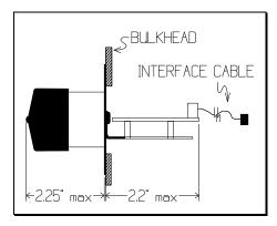
Figure 1: Typical Bulkhead Style Detector Mounting
