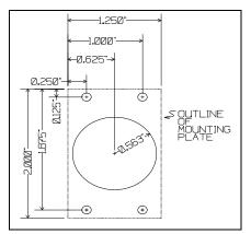
Figure 2: Bulkhead Detector Mounting Pattern
