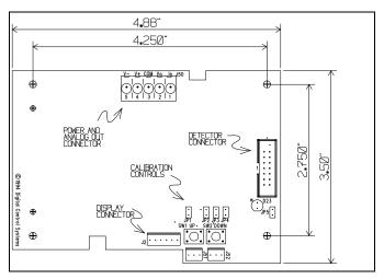
Figure 3: Control Board Layout
