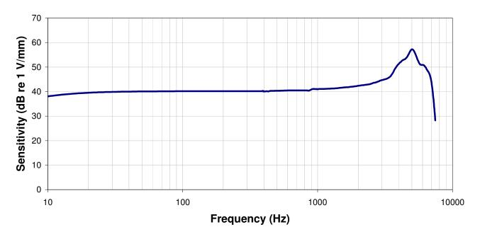
The above plot shows a typical frequency response curve for a device clamped below and subjected to piston-like displacement to the face of the rubber sensing pad.
