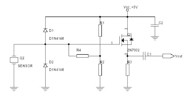
Shield (braid): GND  $C1 = C2 = 0.1 \mu F$ Red wire:  $V_{CC}$ , +5V R1 = R2 = 300 KYellow wire: Vout R3 = 10 K
