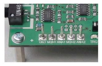
There are five test points with 1.3mm (0.05") pins for measuring the analog voltages evaluated by the microcontroller. The meaning of these voltages is thoroughly explained in paragraph 1.2 on page 4.
