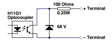
The above schematic shows the internal circuitry of the TRG1 & 2 and AUX1 & 2 optocoupler outputs. When the phototransistor is illuminated by the LED (ON condition) current flows into the + terminal and out of the - terminal. The resistor limits the maximum allowable current to 50mA. Therefore, any DC voltage applied directly to the outputs must not exceed 5V when the phototransistor is conductive because the maximum power the 100 Ohm resistor can dissipate is 250mW.
