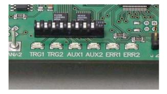
There is a display of six LEDs controlled by the microcontroller. TRG1, TRG2, AUX1 and AUX2 are yellow, and ERR1 and ERR2 are red. Please refer to the software section of this manual for the meaning of the LED signals.
