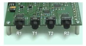
Two fiber optic load sensors can be connected to the MD-220 via four SMA 905 fiber optic receptacles. Viewed from the front the receptacles for Channel 1 are on the left hand side and those for Channel 2 on the right hand side. The transmitters are the inner receptacles.
