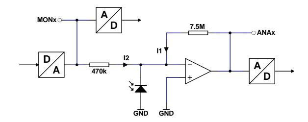
The drawing above is a simple circuit diagram of one channel. When the photodiode is illuminated with light from the sensor it proportionally sinks a current to the incoming light power. This causes the output of the OP to go high so the current is supplied across the 7.5M resistor. When the light becomes too bright the OP output is clipped, and the controller supplies additional current via the DAC and the 470k resistor until the OP output is "unclipped."
