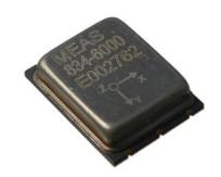
The Model 834 is a low cost, board mountable triaxial accelerometer designed for high amplitude embedded shock applications. The accelerometer features a maximum current consumption of 4 micro-amps and incorporates full power and signal conditioning. The model 834 is available in ±2000g to ±6000g ranges and provides a flat frequency response up to 2kHz. The model 834M1 provides an extended frequency range to 6kHz.
