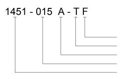
Coating (F = Gel Fill, Blank = No Coating) Port (T = Tube, N = Narrow Hole, W = Wide Hole) Type (A = Absolute, G = Gage) Pressure Range Model
