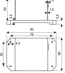
NS-5/V Single Axis Inclinometer With analog voltage output
