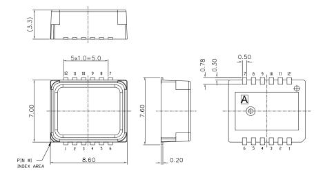
Figure 3. Housing dimensions
