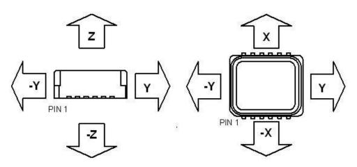
Figure 2. Accelerometer measuring directions
