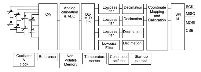
Figure 1. SCA2120-D07 Block diagram
