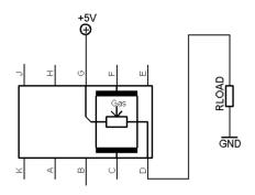
MiCS-2614 with recommended supply circuit (top view)
