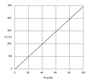
Fig. 4:  $\Delta T$  as a function of P<sub>h</sub>
