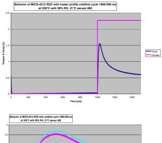
Behavior of MICS-4512 RED with coldhot cycle 1000-500 ms at 350°C with 50% RH, 21°C sensor #22
