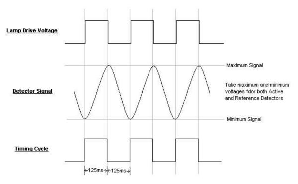
Figure 2 - Measurements in relation to the lamp drive voltage
