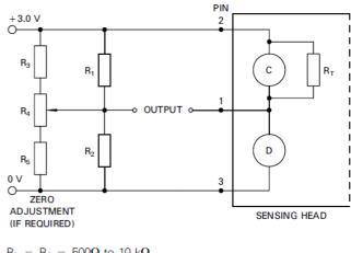
$R_1 = R_2 = 500\Omega$  to 10 k $\Omega$  $R_3 = R_5 \simeq 10R_1$  $R_4 \simeq 20R_1$
