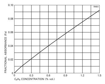
Typical Sensitivity to Acetylene (100% LFL = 2.5% vol.) (IR14BD)
