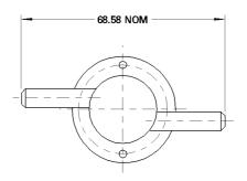
The Quick Calibration Hood is constructed from polypropylene, and provides a convenient means of supplying test gases to the IR600 in the field, for calibration and checking purposes. The assembly push-fits into the central gas access recess of the head, and is designed to accommodate 6 mm ID or 1/4" flexible tubing.
