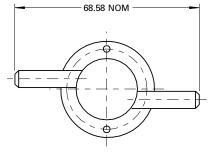
The Quick Calibration Hood is constructed from polypropylene, and provides a convenient means of supplying test gases to the IR600 in the field, for calibration and checking purposes. The assembly push-fits into the central gas access recess of the head, and is designed to accommodate 6 mm ID or 1/4" flexible tubing.
