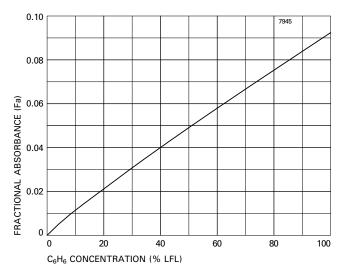
Typical Sensitivity to Acetylene (100% LFL = 2.5% vol.) (IR604)
