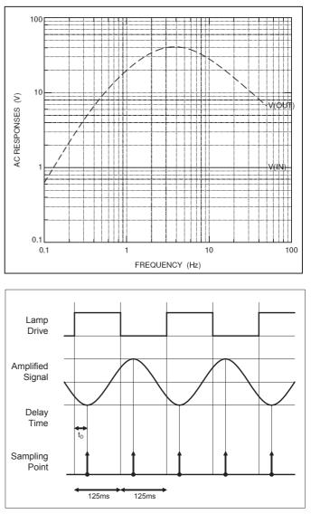
On some sensors where there is a difference in output level between the active and reference channels there will be a difference in delay time for each channel. In this situation the delay time should be set to the average value. The following section explains how to set the ADC measurement delay time and other sensor specific parameters.
