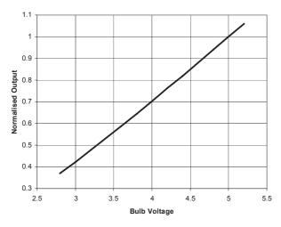
**Pyro Output Voltage vs. Lamp Supply** (IR12GJ Active Channel, Normalised at 5.0 V)
