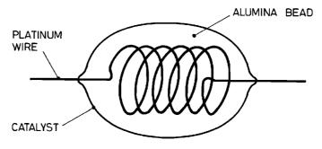
The design has been modified to reduce the amount of power used by the sensor and to make the sensor more resistant to poisoning and mechanical shock. e2v, when known as EEV, was in the forefront of these developments and the current range of pellistors incorporates the design improvements.
