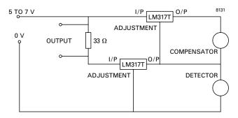
Note: Voltage across compensator and voltage across detector  $\simeq$  1.25 V.
