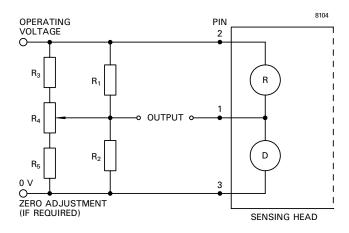
$R_1 = R_2 = 500 - 2000 \Omega,$  $R_3 = R_5 \simeq 10R_1, R_4 \simeq 20R_1$
