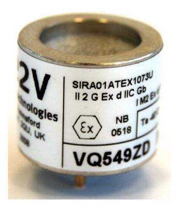
For the VQ549ZD/W, a carefully matched set of detector, compensator and resistor are encapsulated in a cylindrical stainless steel housing with an integral stainless steel sinter at one end to permit the entry of the atmosphere. Electrical connections are made to three pins at the other end of the body.
