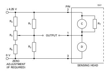
$R_1 = R_2 = 500\Omega$  to 10 k $\Omega$   $R_3 = R_5 \simeq 10R_1$  $R_4 \simeq 20R_1$
