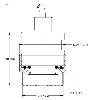
The Weather Cap protects the VQ600 from water when used in external locations, where rain or spray could interfere with the safe working of the head, or in internal locations where water jets, sprays or hoses are used routinely for cleaning purposes, etc. The cap is made of 316 stainless steel and has been tested to IP64 for effectiveness, and also to ensure that it does not significantly affect the VQ600's performance.
