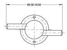
The Quick Calibration Hood is constructed from polypropylene, and provides a convenient means of supplying test gases to the VQ600 in the field, for calibration and checking purposes. The assembly push-fits into the central gas access recess of the head, and is designed to accommodate 6 mm ID or  $^{1}$ /<sub>4</sub>" flexible tubing.
