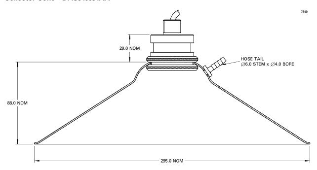
The Collector Cone is designed to enhance the performance of the VQ600 when used in applications involving the detection of leaks of gases which are lighter than air, such as hydrogen or methane. Easily fitted to the VQ600 via the external M46 thread, the assembly collects rising gases and directs them to the VQ600 for maximum detection sensitivity. The painted spun
