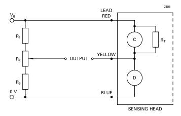
$\rm R_1=R_3=500~to~5000~\Omega,~~R_2\simeq R_1/5$   $\rm R_2$  provides zero adjustment and may be omitted if not required.
