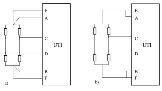
Figure 13. Connection of the resistive bridge to the UTI for the Ub2 mode in a 4-wire setup (a) and a 2-wire setup (b).
