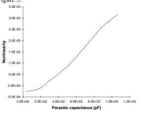
Figure 5 The nonlinearity versus the parasitic capacitance  $C_p$ . The measurement range equals 0 - 2 pF.
