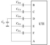
Figure 6. Connection of capacitors to the UTI.
