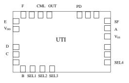
Figure 17 The pad configuration of UTI chip.
