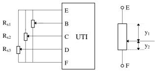
Figure 16. Connection of potentiometers to the UTI.
