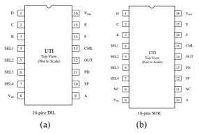
Figure 1 Pin configuration.
