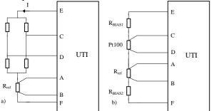
Figure 14. Connection of the resistive bridge and a reference resistor to the UTI (a) and connection of a platinum resistor in 4-wire setup (b).
