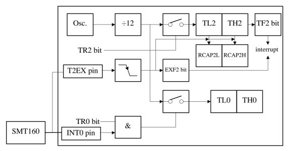
Figure 4. Duty-cycle measurement with Timer 2 and Timer 0.
