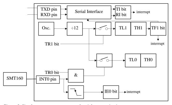
Figure 3. Simultaneous measurement and serial communication
