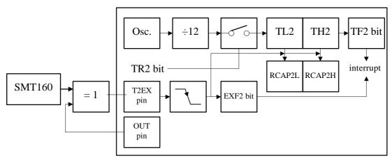
Figure 5. Duty-cycle measurement using Timer 2 only.
