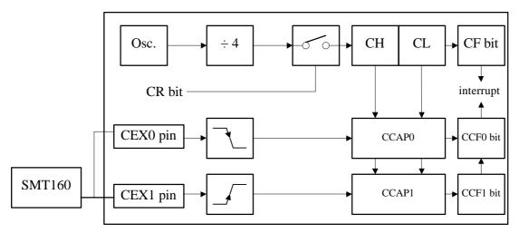
Figure 6. Duty-cycle measurement using the PCA.
