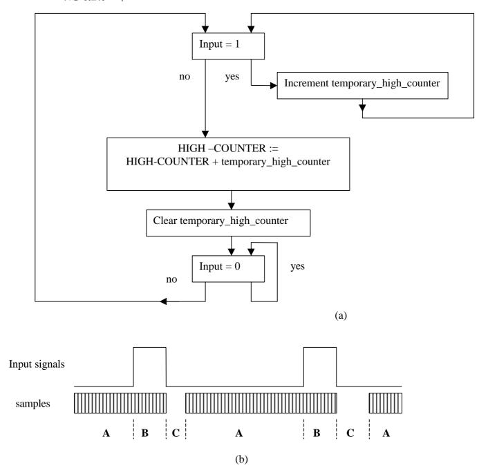
Figure 7 a) Flow diagram of a duty-cycle measurement by software (only the part to measure the "high"-time).
