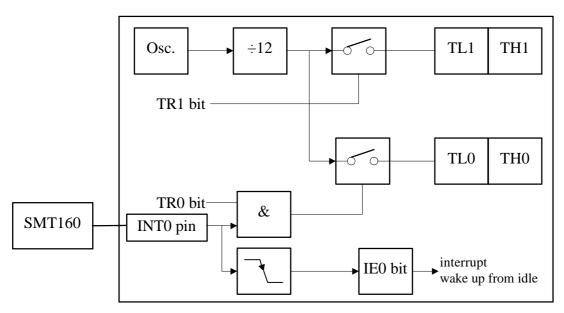
Figure 1. Configuration of internal 8051 hardware
