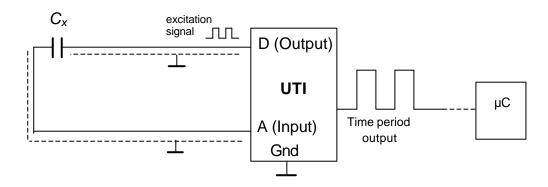
Fig. 3 Practical UTI connection (measuring C<sub>x</sub> only)
