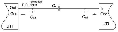
Fig.2 Two-port UTI approach (measuring C<sub>x</sub> only)
