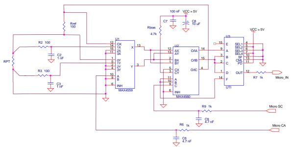
Figure 3 A testing circuit diagram.
