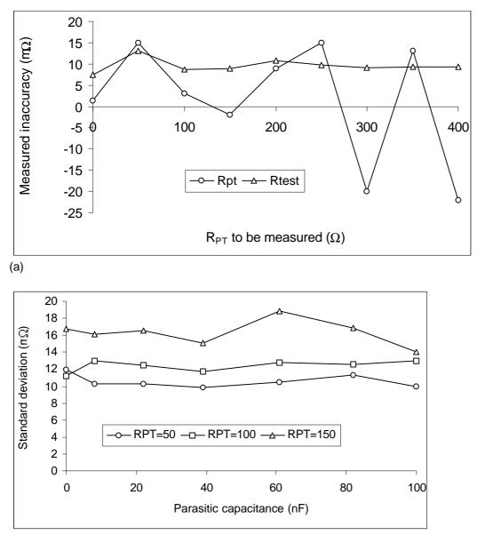
Figure 5 The effect of parasitic capacitance on the measurement of  $R_{PT}$ , a) accuracy, b) standard deviation.
