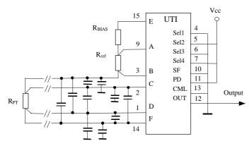
Figure 1 The parasitic capacitors effect.
