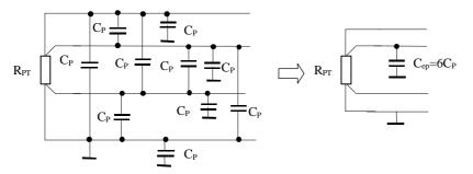
Figure 4 An equivalent model of long cable wire.
