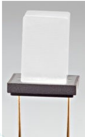
Crystal coupled directly to a sensL SPM
